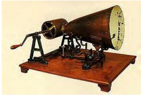
Leon De Martinville's Phonautograph 1857. From the Smithsonian Collection. The first instrument to record sound.
