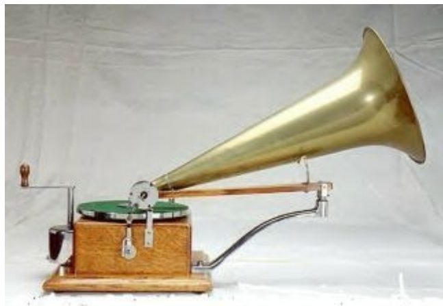
Berliner's 1896 Improved Gramophone with Johnson's Spring-Wound Motor
