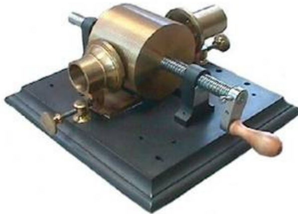
Edison's Tin-Foil Cylinder Phonograph The original instrument was fabricated by John Kruesi in Edison's Laboratory during December 2-6, 1877
